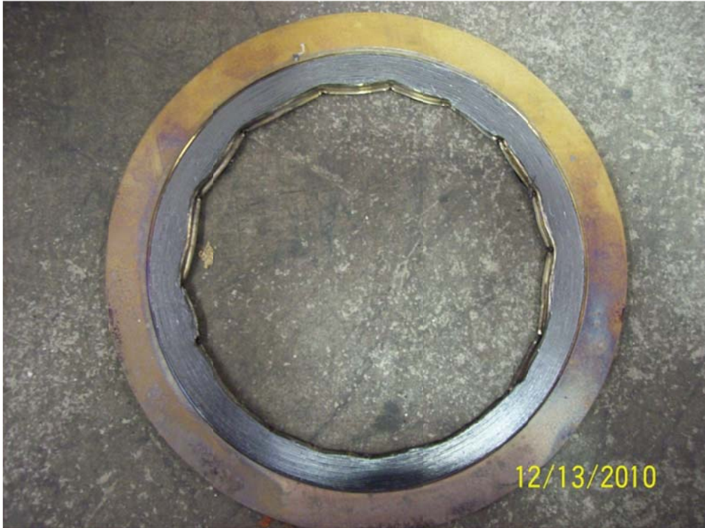
Gasket After Test
