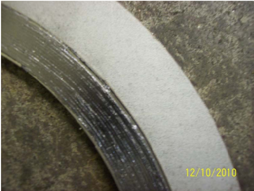
Gasket Before Test
